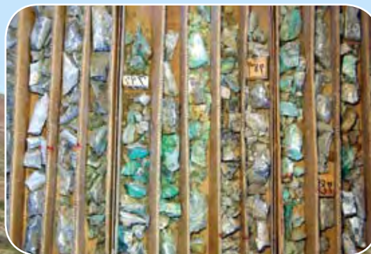
Gunnison drill core showing copper oxide mineralization
